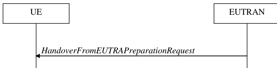
Figure 5.4.4.1-1: Handover from E-UTRA preparation request
