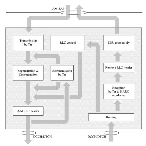
Figure 4.2.1.3.1-1: Model of an acknowledged mode enttiy
