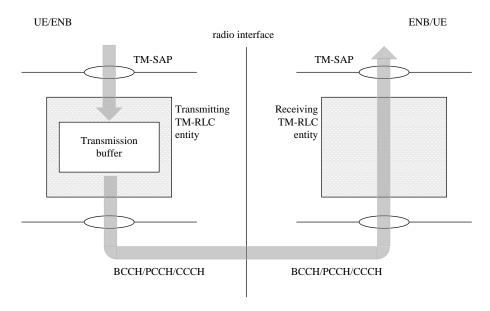
Figure 4.2.1.1.1-1: Model of two transparent mode peer entities
