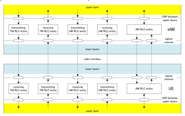
Figure 4.2.1-1: Overview model of the RLC sub layer
