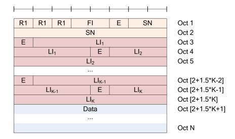
Figure 6.2.1.3-6: UMD PDU with 10 bit SN (Even number of Lls, i.e. K = 2, 4, 6, ...)
