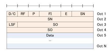
Figure 6.2.1.5-1: AMD PDU segment (No LI)
