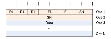
Figure 6.2.1.3-2: UMD PDU with 10 bit SN (No LI)
