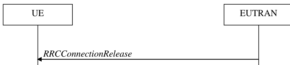
Figure 5.3.8.1-1: RRC connection release, successful
