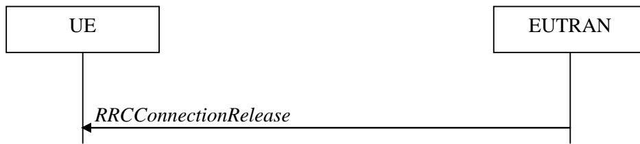
Figure 5.3.8.1-1: RRC connection release, successful
