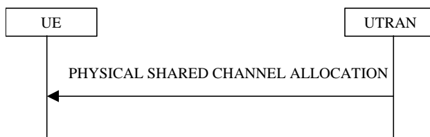
Figure 8.2.7-1: Physical Shared Channel Allocation
