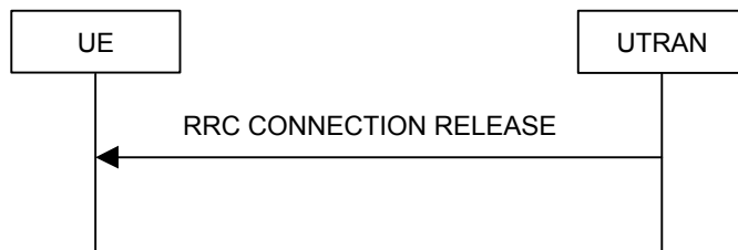
Figure 8.1.4-2: RRC Connection Release procedure on the CCCH
