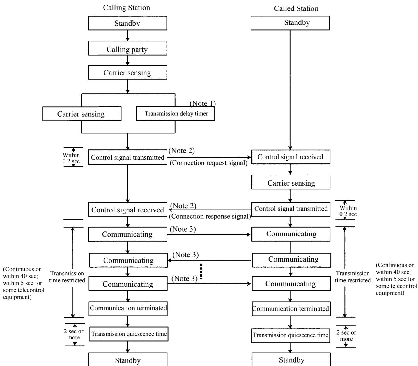
Figure 3.3 Example of the Channel Connection Procedure in a Simplex Operation (Fixed and Manual Channel Switching)
