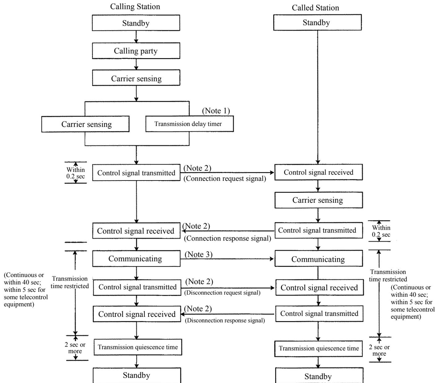
Figure 3.4 Example of the Channel Connection Procedure in Semi-duplex and Duplex Operation (Fixed and Manual Channel Switching)
