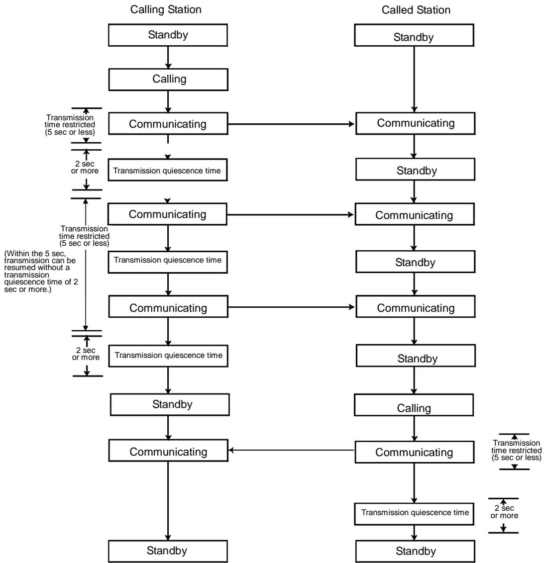
Figure 3.1 Sample Transmission Times in a Simplex Operation
