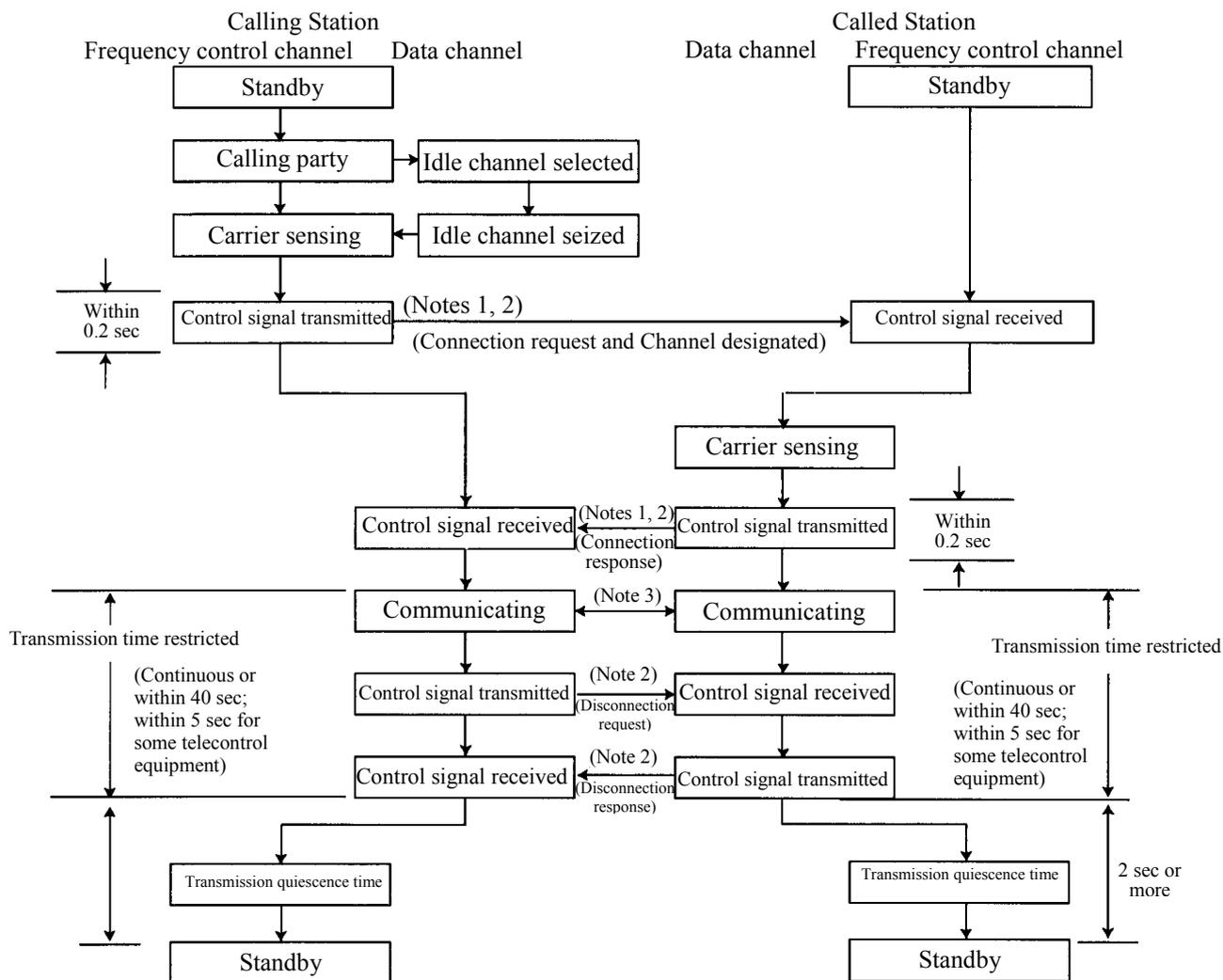
Figure 3.5 Example of the Channel Connection Procedure in Semi-duplex and Duplex Operation (Automatic Channel Switching through the Frequency Control Channel)
