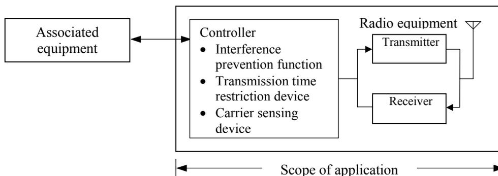
Figure 1.1 Configuration of Telemetry, Telecontrol and Data Transmission Radio Equipment
