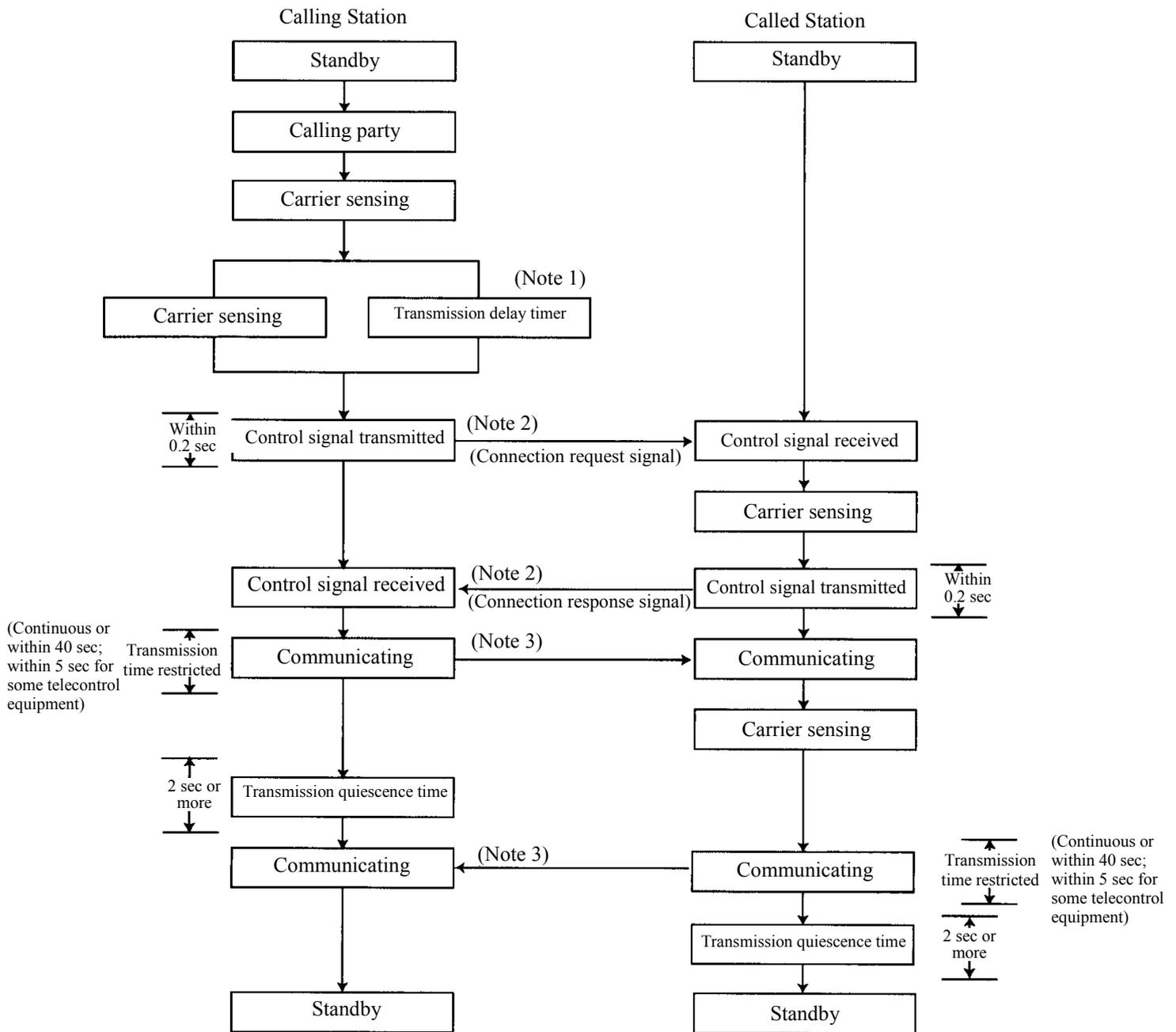
Figure 3.2 Example of the Channel Connection Procedure in a Simplex Operation (Fixed and Manual Channel Switching)
