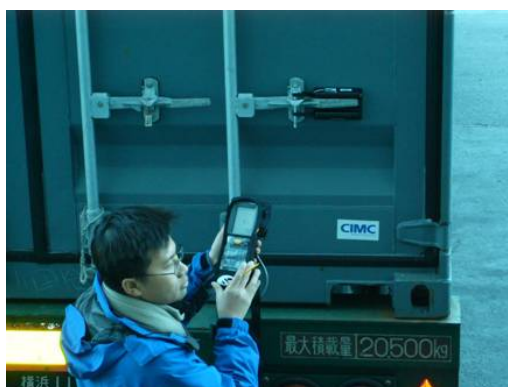
Figure 2-6 A use scene of a 433MHz-band transportable interrogator at a storehouse
