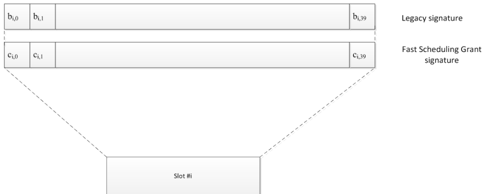
Figure 5.4.3.2.3-1. Re-using E-RGCH for fast scheduling grant
