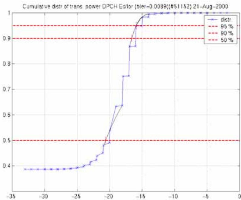
Figure 57: Distribution of transmission power DPCH_Ec/Ior when compressed mode is on. TGL = 7 slots. The gap in the PDF probably exists because of the bin widths
