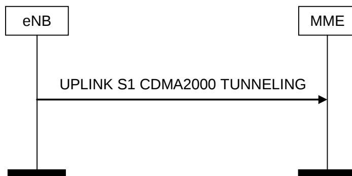
Figure 19.2.2.16.2-1: Uplink S1 CDMA2000 Tunneling procedure
