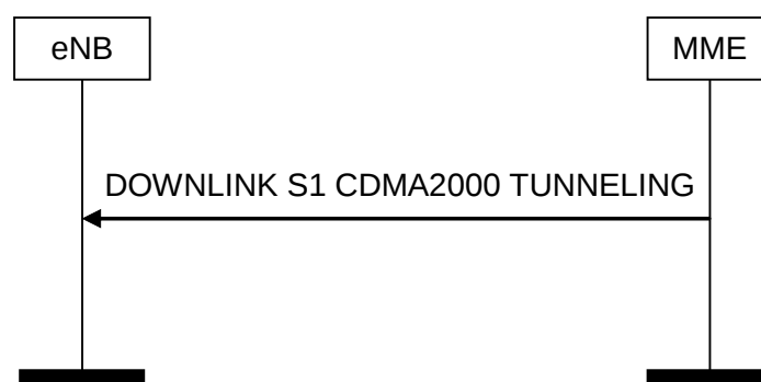
Figure 19.2.2.16.1-1: Downlink S1 CDMA2000 Tunnelling procedure
