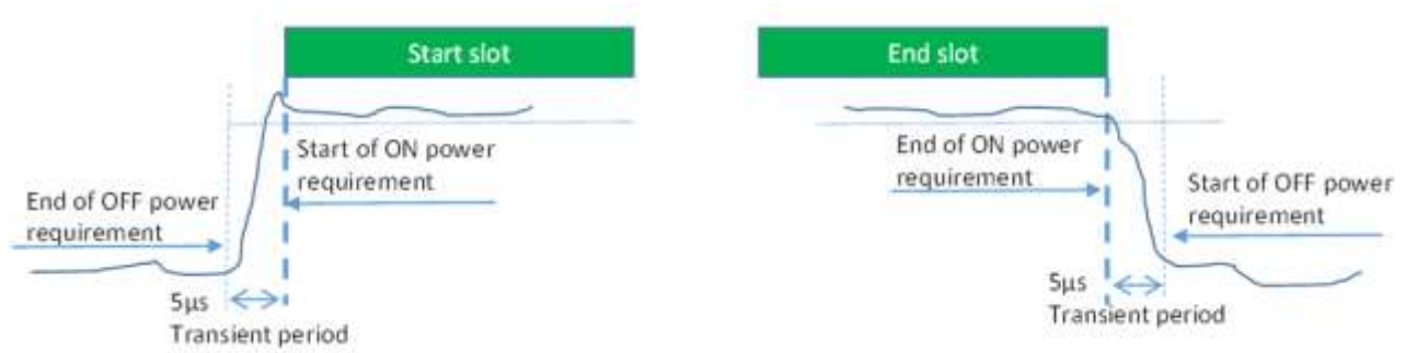
Figure 6.3.3.2-1: General ON/OFF time mask for NR UL transmission in FR2
